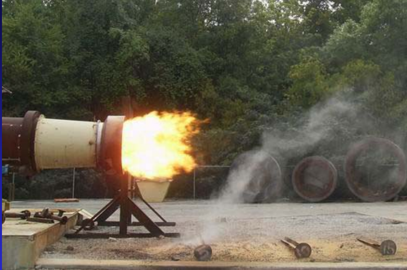
ASTEC prototype, @ 42 MM Btu/hr
